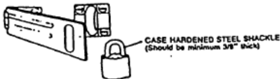
A HEAVY DUTY PADLOCK (3/8" Case hardened steel shackle) FIVE PIN TUMBLER OPERATION
